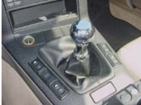
Install AA Signature Shift Knob using allen screws to secure.
