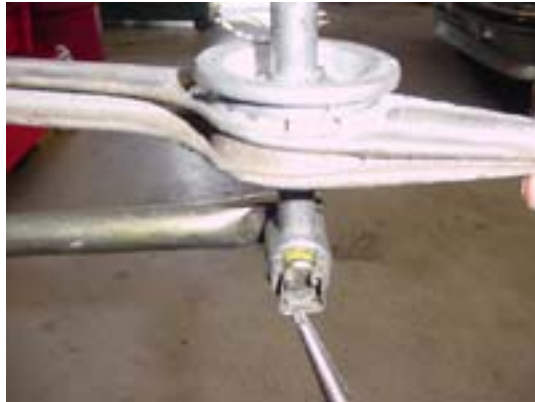
Look for the end of the gear shift lever and connect to shift rod. Secure with the circlip at the end
