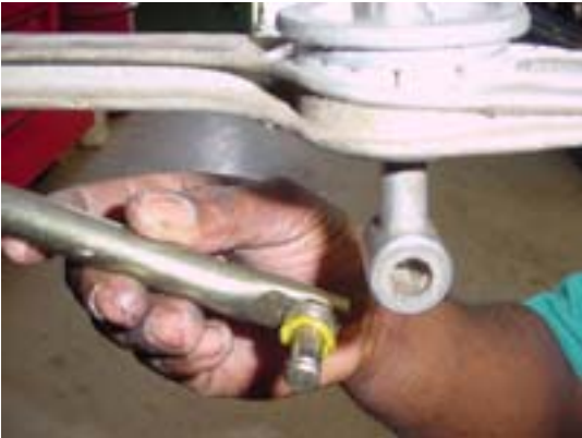
Place the corresponding YELLOW circular washers before connecting to gear shift lever.
