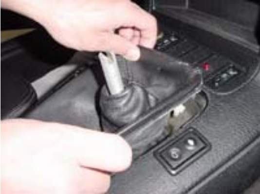
Reinstalling the Gear Shift Boot
